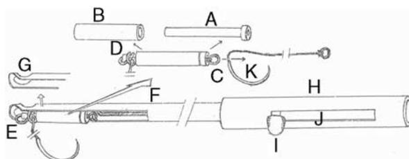
**FIGURE 1.** Components of the novel pusher device: collar tubule (A); outer sheath (B); tiny metallic ring (C); pretied 2-turn slip knot (D); loop formation (E); sleeve (F); hole in the round tip (G); handle (H); control button (I); groove for sliding button (J); metallic wire (K).
