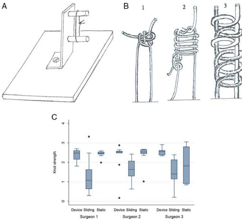
**FIGURE 3.** A, An erect metallic rectangular plate with 2 vinyl-coated screws. B, Double sheet bend (left) for the device group, 4s modified Roeder sliding knot (middle) for the sliding group, and static surgeon's knot (right) for the static group. C, Knot strengths among different surgeons and groups.
